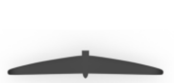
stabilizer span 410 / area 170cm 2
