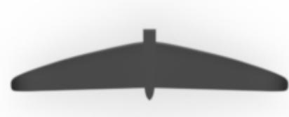
stabilizer span 480 / area 285cm 2
