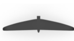
stabilizer span 380 / area 190cm 2
